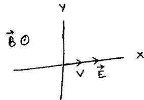
$$\vec{F}_B = q \times \vec{B} (-\hat{j}) \quad \text{using right hand rule.} \\ = 1.80 \mu C \times 3.00 \times 10^6 \frac{m}{s} \times 1.50 \times 10^{-3} T (-\hat{j}) = -8.1 \times 10^{-3} N \hat{j}$$
