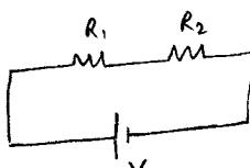
$$(b) I_1 = I_2 = I = \frac{V}{R_{\text{eq}}} = \frac{10.0}{30.0} = 0.333 \text{ A}$$
