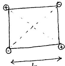
$$(b) V_{\text{side}} = +\frac{ke}{\frac{L}{2}} - \frac{ke}{\frac{L}{2}} + \frac{ke}{\sqrt{\frac{L^2 + \frac{L^2}{4}}{4}}} - \frac{ke}{\sqrt{\frac{L^2 + \frac{L^2}{4}}{4}}} = 0$$
