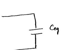
$$C_{eq} = C_1 + C_6 \\ = 1.0 \mu F + 1.56 \mu F \\ = 2.6 \mu F$$
