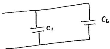
$$\frac{1}{C_6} = \frac{1}{C_2} + \frac{1}{C_S} = \frac{1}{2 \times 7} + \frac{1}{7 \times 2} \\ = \frac{9}{14}$$
