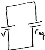
$$\frac{1}{C_{eq}} = \frac{1}{C_1} + \frac{1}{C_{23}} = \frac{1}{10 \times 5} + \frac{1}{50} = \frac{6}{50} \Rightarrow C_{eq} = \frac{50.0}{6} = 8.33 \mu F$$
