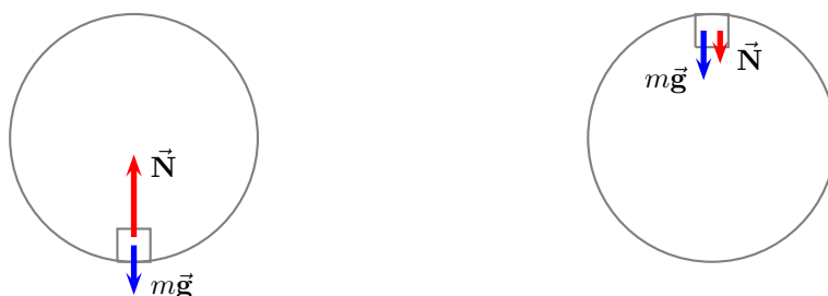
Figure 7.9: Forces acting on a mass while moving in a vertical circle inside a globe.
