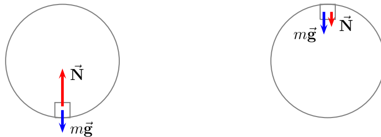
Figure 3: Forces acting on a mass while moving in a vertical circle inside a globe.
