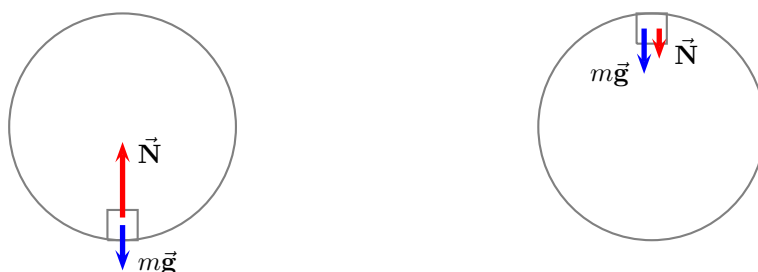
Figure 9.8: Forces acting on a mass while moving in a vertical circle inside a globe.
